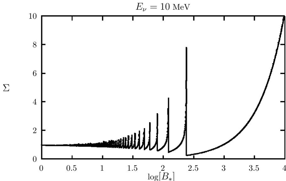
**Figure 1:** Normalised cross section,  $\Sigma \equiv \sigma/\sigma_0$ , for  $E_\nu = 10$  MeV, as a function of the magnetic field  $B_* \equiv B/B_c$ , in the absence of background matter and for  $T = 0$ .
