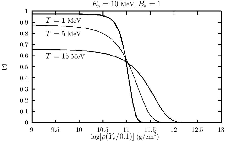
**Figure 3:** Temperature dependence of the  $\Sigma$  vs.  $\rho$  relation, fixing  $E_\nu = 10$  MeV and  $B_* = 1$ .
