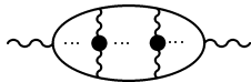
Figure 1. Typical ladder diagram that contributes to the electrical conductivity at leading-logarithmic order. The side rails represent hard nearly on-shell fermions, dressed with a width, and the rungs are soft (HTL resummed) photons.
