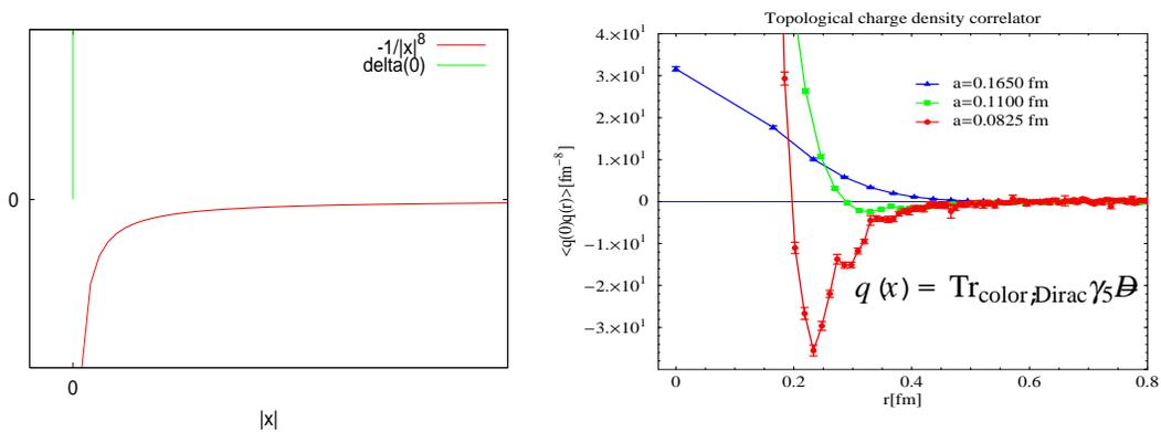
**FIGURE 8.** Correlator of the topological charge density: (left) as expected in the continuum and (right) as measured on the lattice [11]. The negative part and divergent contact term both become visible as  $a \rightarrow 0$ .
