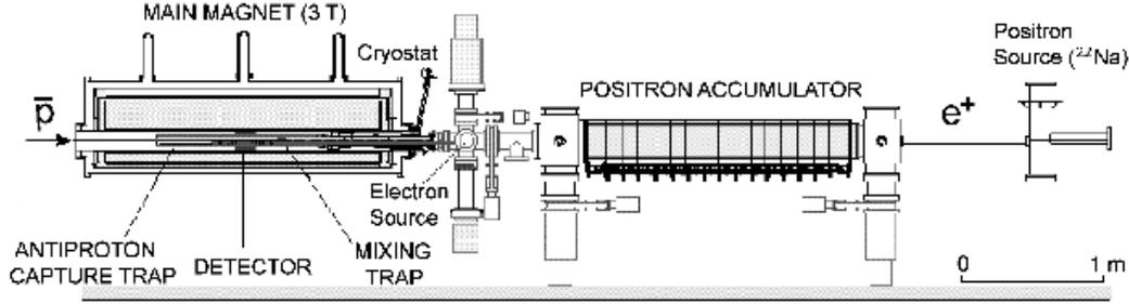
Figure 1. Scheme of the ATHENA apparatus for the production and detection of antihydrogen.
