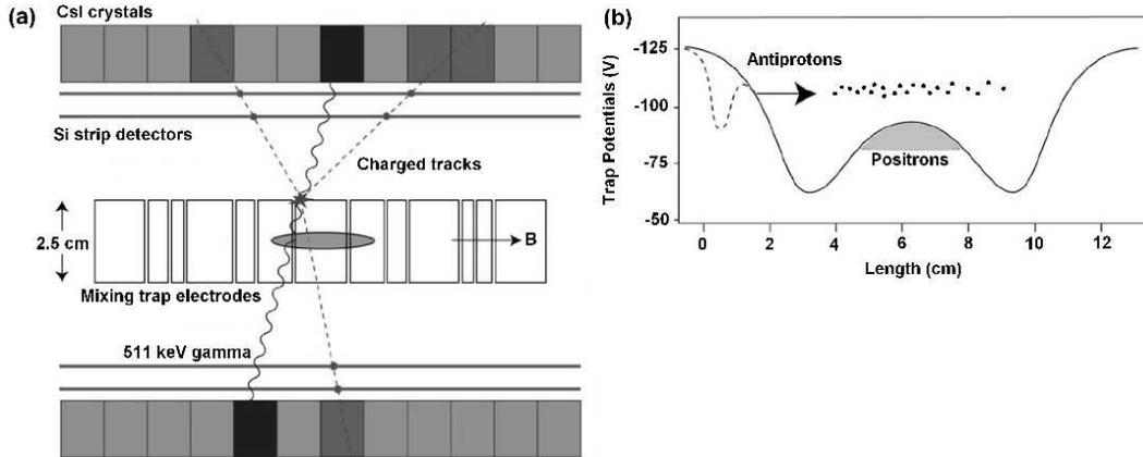
Figure 2. (a) Schematic diagram, in axial section, of the ATHENA mixing trap and  $\bar{H}$  detector with a typical annihilation event. (b) The trapping potential on the axis of the mixing trap is plotted against length along the trap. The dashed line is the potential immediately before antiproton injection while the solid line is the potential during mixing.
