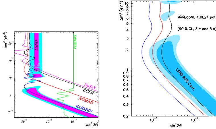
Fig. 1. Left:  $\sin^2 2\theta - \Delta m^2$  plot showing the parameter regions describing the LSND observation (purple, blue). Exclusion curves from various other experiments are shown as well, with the region on the right side excluded (from <sup>4</sup>). Right: In case of a non-observation of an effect in MiniBooNE the regions on the right side of the curves can be excluded with the shown significance.
