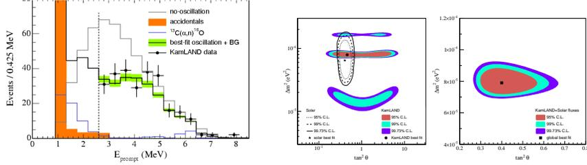
Fig. 4. Left: Prompt energy spectrum as observed by KamLAND. A clear spectral distortion can be seen. Right: Combined KamLAND and solar data fits (from <sup>11</sup>).
