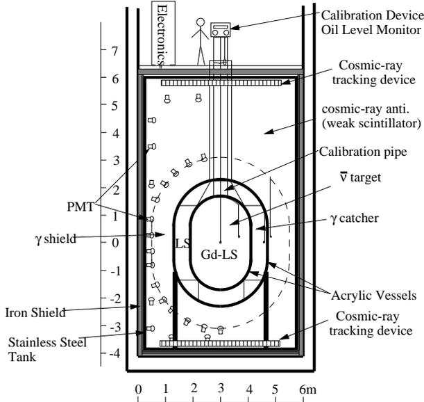
Figure 1. Schematic view of the KASKA detector.
