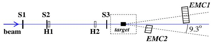
**Figure 1.** Experimental Setup PROZA-M. S1-S3 – trigger scintillation counters; H1-H2 – hodoscopes; EMC1 and EMC2 – electromagnetic calorimeters; *target* – polarized target.
