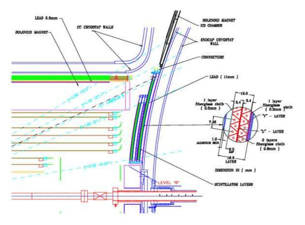
Figure 5: The central and forward preshower detectors, with a detail of the FPS construction.
