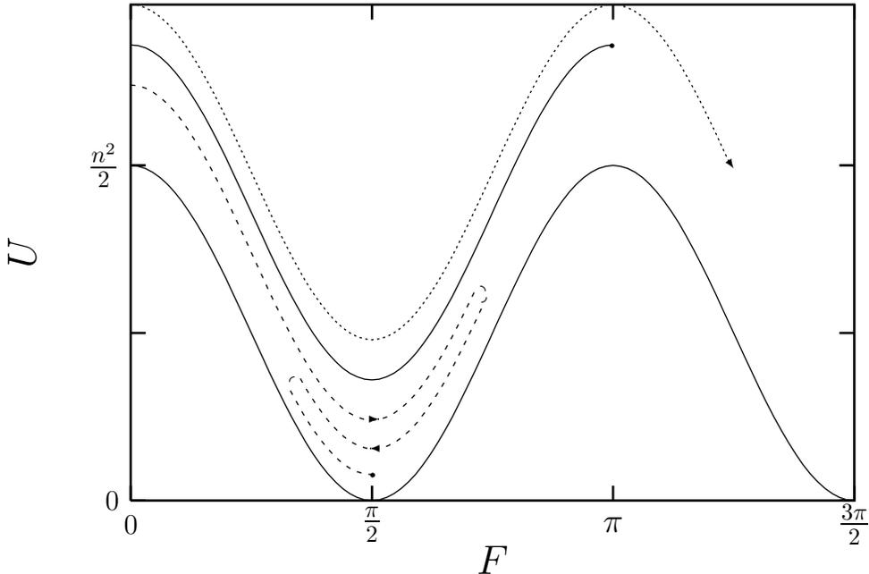
FIG. 1. Shape of the effective potential  $U$  and possible motions of a hypothetical particle: (a) overshoot solution (the dotted line), (b) critical solution with  $F(\infty) = \pi$  (the solid line), (c) undershoot solution with  $F(\infty) = \pi/2$  (the dashed line).
