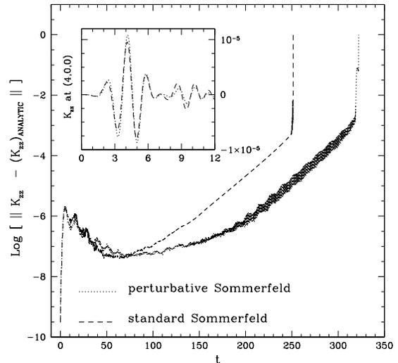
FIG. 4. Long-term evolution of the  $L_2$  norm of the error in  $K_{zz}$  at the 3D outer boundary surface. The inset shows  $K_{zz}$  at the outer boundary along the  $x$ -axis. The interior grid has  $(33)^3$  gridpoints and the code is stopped when the norm is unity.
