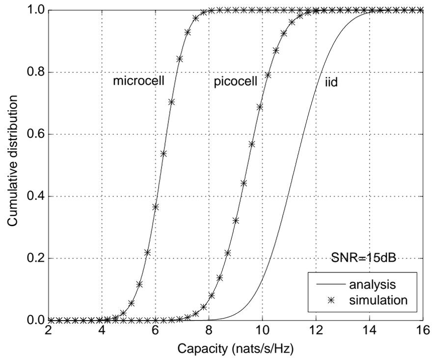
Fig. 7. CDF of the capacity for doubly correlated MIMO channels with  $n_T = n_R = 4$  and METRA correlation matrices given in [?, p. 82] for picocell and microcell environments. For comparison, the CDF of capacity for the  $4 \times 4$  i.i.d. MIMO channel is also plotted.  $\eta = 15$  dB.
