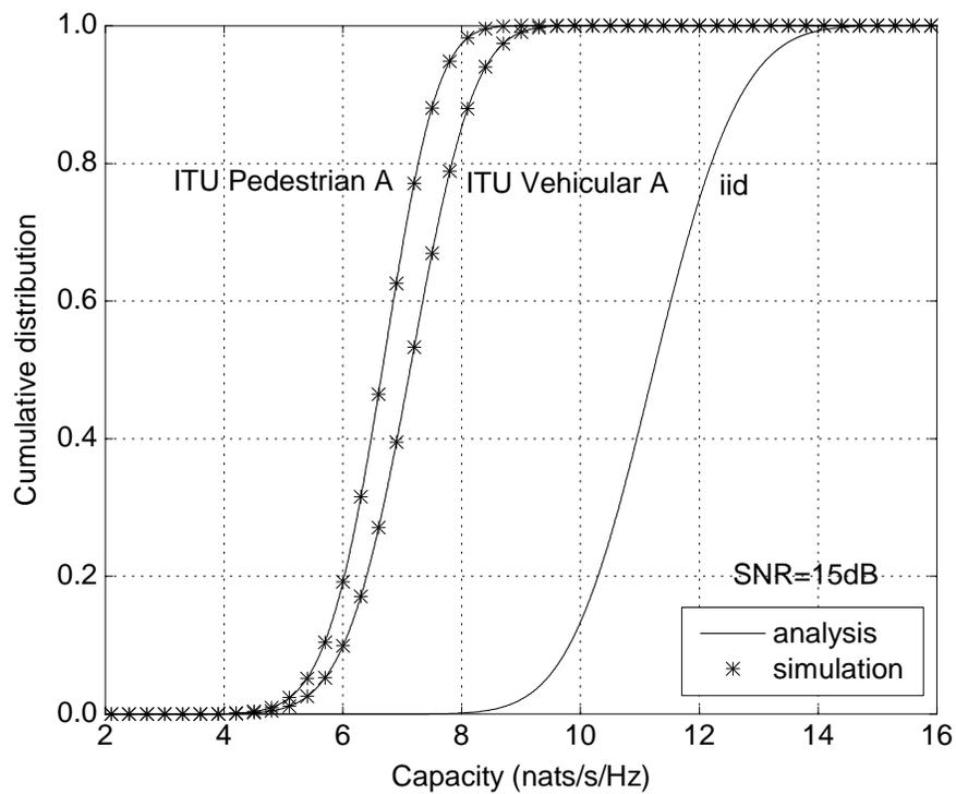
Fig. 9. CDF of the capacity for doubly correlated MIMO channels with  $n_T = n_R = 4$  and METRA correlation matrices given in [?] for macrocell ITU Pedestrian A and Vehicular A environments. For comparison, the CDF of capacity for the  $4 \times 4$  i.i.d. MIMO channel is also plotted.  $\eta = 15$  dB.
