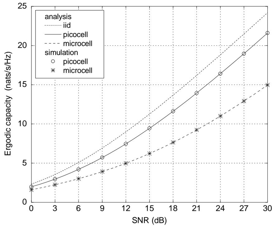
Fig. 6. Ergodic capacity of doubly correlated MIMO channels with  $n_T = n_R = 4$  and METRA correlation matrices given in [?, p. 82] for picocell and microcell environments. For comparison, the ergodic capacity of the  $4 \times 4$  i.i.d. MIMO channel is also plotted.
