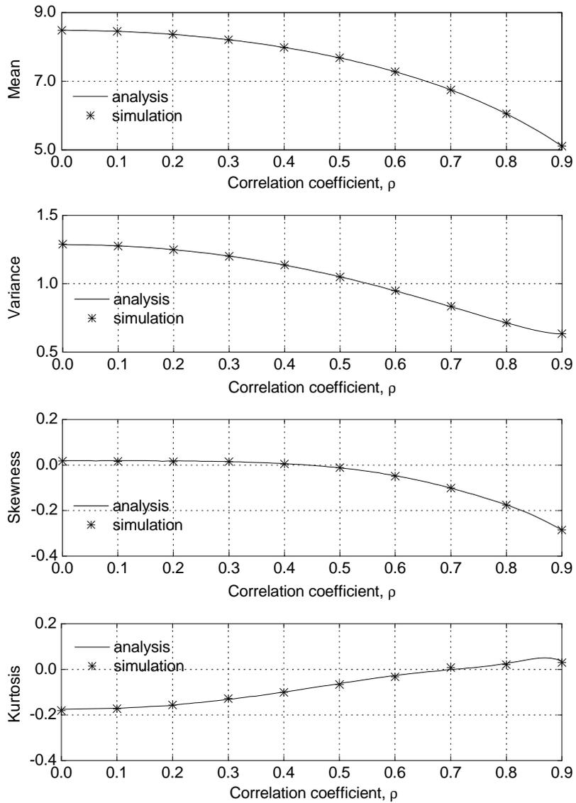
Fig. 4. Mean, variance, skewness, and kurtosis of the capacity (nats/s/Hz) as a function of correlation coefficient  $\rho$  for exponentially correlated MIMO channels with  $\rho_T = \rho_R = \rho$ .  $n_T = n_R = 3$  and  $\eta = 15$  dB.
