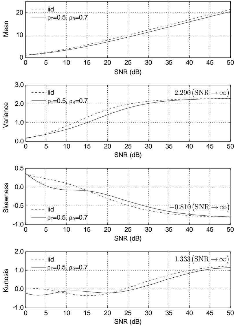
Fig. 5. Mean, variance, skewness, and kurtosis of the capacity (nats/s/Hz) versus SNR for i.i.d. and doubly correlated ( $\rho_T = 0.5$ ,  $\rho_R = 0.7$ ) MIMO channels.  $n_T = n_R = 2$ .
