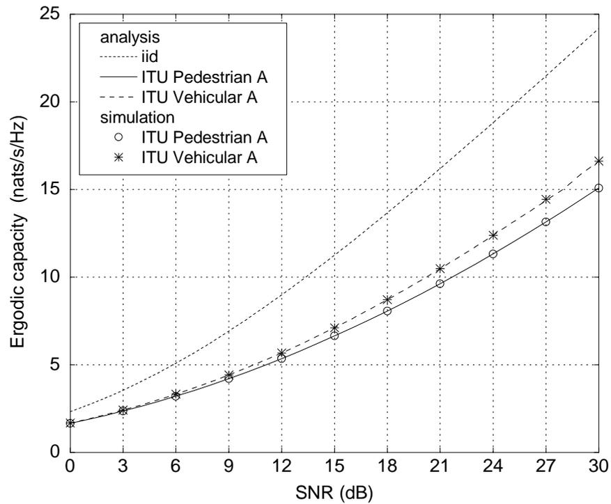
Fig. 8. Ergodic capacity of doubly correlated MIMO channels with  $n_T = n_R = 4$  and METRA correlation matrices given in [?] for macrocell ITU Pedestrian A and Vehicular A environments. For comparison, the ergodic capacity of the  $4 \times 4$  i.i.d. MIMO channel is also plotted.
