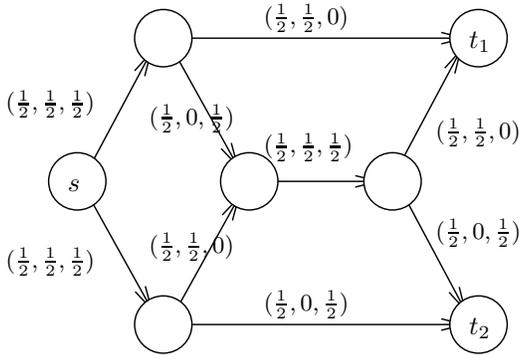
(b) Each arc is marked with the triple  $(z_{ij}, x_{ij}^{(1)}, x_{ij}^{(2)})$ .
