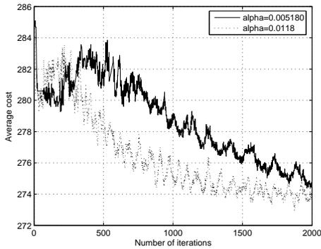
Fig. 3. Average energy of a random 4-terminal multicast of unit rate in a 30-node wireless network using the primal-dual method of Section II-B. Nodes were placed randomly within a  $10 \times 10$  square with a radius of connectivity of 3. The energy required to transmit at rate  $z$  to a distance  $d$  was taken to be  $d^2 e^z$ . Source and sink nodes were selected according to a uniform distribution over all possible selections.
