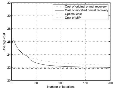
Fig. 2. Average energy of a random 4-terminal multicast of unit rate in a 30-node wireless network using the subgradient method of Section II-A. Nodes were placed randomly within a  $10 \times 10$  square with a radius of connectivity of 3. The energy required to transmit at rate  $z$  to a distance  $d$  was taken to be  $d^2 z$ . Source and sink nodes were selected according to a uniform distribution over all possible selections.
