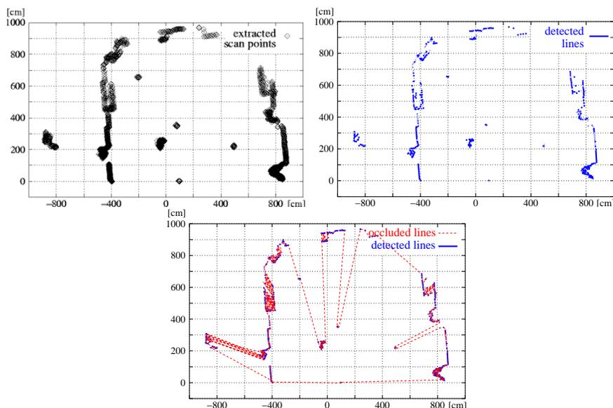
**Fig. 8.** A typical scenario faced by Kurt3D. Top left: Extracted points at height 75 cm (corresponding to figure 1, bottom middle). Top right: Line detection using Hough transform. Bottom: Automatically generated map with occlusion lines [16].
