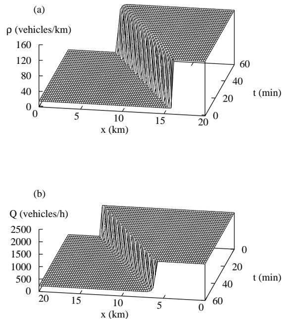
FIG. 10. Simulation of an upstream front with initial densities of  $\rho_1 = 15 \text{ vehicles/km}$  and  $\rho_2 = 140 \text{ vehicles/km}$ . Shown is the spatio-temporal evolution of (a) the density, and (b) the flow. In (b), the direction of the space and time axes is reversed for illustrative reasons.
