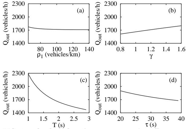
FIG. 12. Outflow  $Q_{\text{out}}$  from a congested traffic state of density  $\rho_1$  in dependence of (a)  $\rho_1$ , (b)  $\gamma$ , (c)  $T$ , and (d)  $\tau$ . The simulated traffic situation is that of Fig. 11. The outflows were determined after a transient time of 30 minutes.
