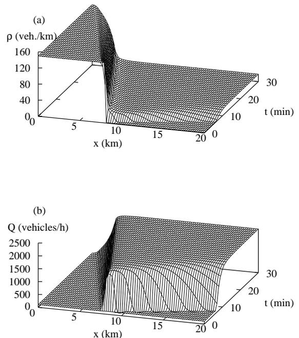
FIG. 11. Simulations of downstream-fronts with  $\rho_{\text{jam}} = 140$  vehicles/km. Shown is the spatio-temporal development of (a) the density, and (b) the flow. Free boundary conditions were used on both sides.
