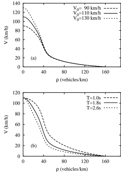
FIG. 3. Variation of the equilibrium velocity-density relation of the GKT model with (a) the desired velocity  $V_0$ , and (b) the safe time headway  $T$ . The other parameters have the standard values displayed in Table I.
