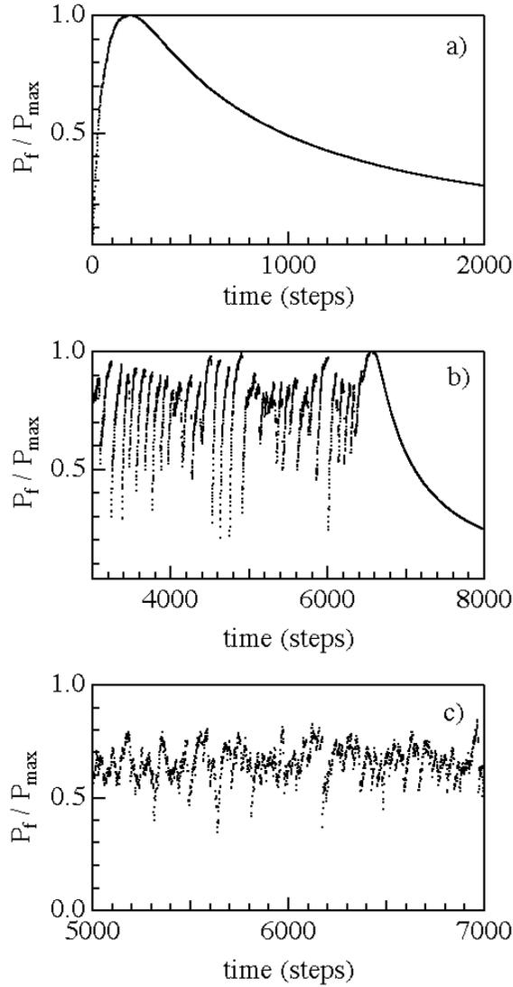
FIG.6 Three examples of model-generated evolution curves. All parameters are the same except the growth rate ( $STEP$ ) of the dissipative elements. This parameter has the value  $STEP = 0.2/NR_s$ ,  $0.3/NR_s$ , and  $0.6/NR_s$  for curves a), b), and c), respectively. The other parameters are  $N = 80$ ,  $N_1 = 5$ , and  $P_c = 1.8P_{max}/N$ .
