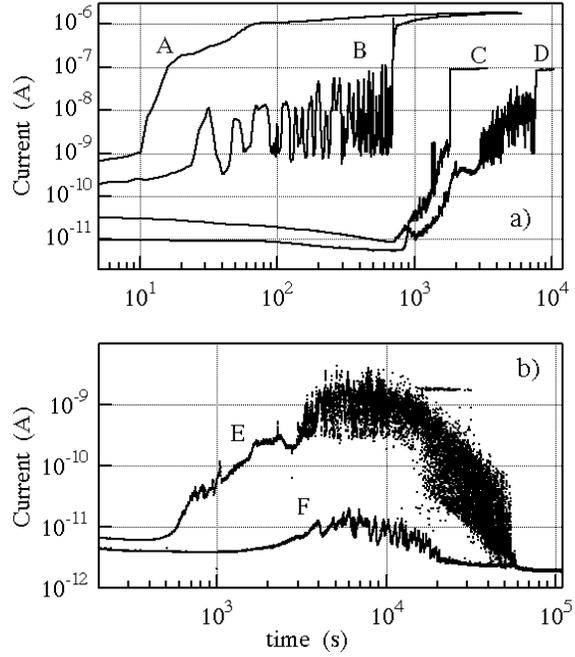
FIG.3 Examples of the evolution curves (current vs time) for two samples. (a) The curve B is measured after the curve A on the same sample with  $R_s = 48.1M\Omega$  and  $V_0 = 100V$ . Curves C, D, E, and F show successive runs on another sample with  $R_s = 1.04G\Omega$  and  $V_0 = 100V$  (curves E and F are plotted in the part (b)). The particle concentration was  $\approx 0.02mg/ml$  in all cases.
