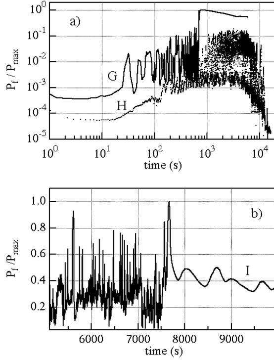
FIG.4 The total power dissipated by the fluid  $P_f = IV_f$ , normalized by the maximum power  $P_{max} = V_0^2/4R_s$ , is plotted vs time. The curves G and I are derived from curves B and D (Fig.3) respectively. The curve H is calculated from an  $I(t)$  curve measured after the curve B.
