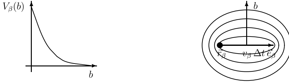
Fig. 1: Left: Decrease of the repulsive interaction potential V_\beta(b) with b . Right: Elliptical equipotential lines of V_\beta[b(\vec{r} - \vec{r}_\beta)] for different values of b .
