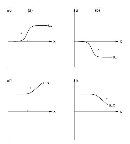
FIG. 10. In a) and b) we show right and left-moving solitons with vanishing amplitude at x = -L/2. The associated height profiles correspond to the bottom and top part of a step, respectively (arbitrary units)..
