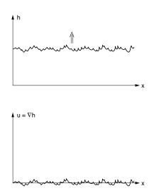
FIG. 1. We depict the general growth morphology for a 1-D interface in terms of the slope field u and the height field h (arbitrary units).
