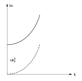
FIG. 4. We show the diffusive dispersion law in the presence of a soliton. The gap in the spectrum is given by  $\nu k_s^2 = \lambda^2 u_+^2/4\nu$  where  $u_+$  is the soliton amplitude. The dashed line indicates the gapless spectrum in the linear case (arbitrary units).
