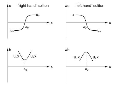
FIG. 8. In a) and b) we show the static *right* and *left hand* solitons and the smoothed static downward and upward cusps in the associated height field (arbitrary units).
