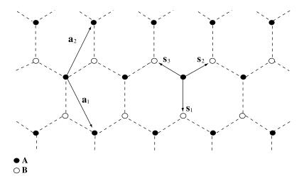
Figure 1: Graphene hexagonal lattice constructed as a superposition of two triangular lattices A and B, with basis vectors  $a_i$  for lattice A and vectors  $s_i$  connecting A to B.
