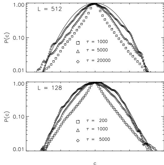
FIG. 4: Distributions of coefficient of wavelets transform at three time scales. The heights of the PDFs have been scaled to their maximum value, and the widths to the standard deviation. The solid curve is a Gaussian with the same amplitude and variance, plotted for reference. Upper plot, the lattice length is  $L = 512$ ; lower plot, for comparison,  $L = 128$ .
