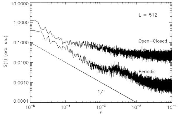
FIG. 2: Power spectrum of the synthetic signal for both periodic and open-closed boundary conditions. Overplotted for comparison is a  $1/f$  curve.
