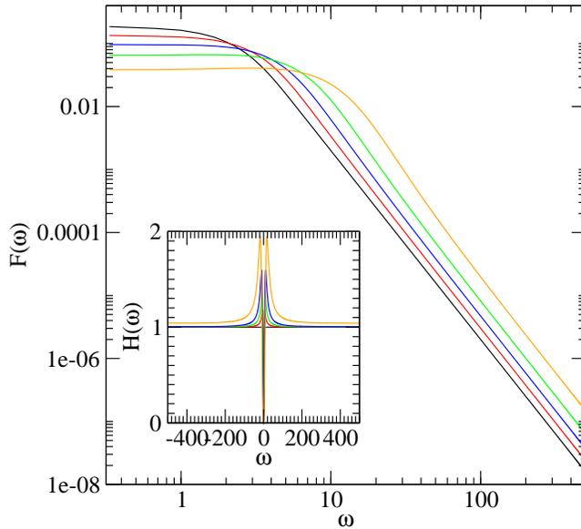
Fig. 3 – Log-Log plot of  $F(\omega)$  of the “zero mass” needle with different values of the coefficient of restitution  $\alpha = 0, 0.2, 0.4, 0.6, 0.8$  from top to bottom. The inset shows the  $\omega$ -dependence of the rescaled function  $H(\omega) = F(\omega) \frac{mL^2(1-\alpha)}{4T(1+\alpha)} \omega^3$  for  $T/(mL^2) = 1/2$ .
