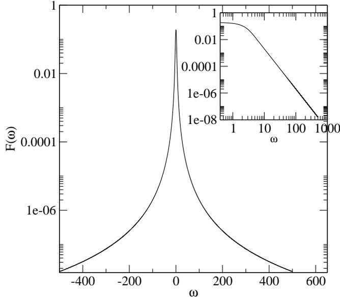
Fig. 2 – Log-linear plot  $F(\omega)$  of the “zero mass” needle. The inset displays the log-log plot showing the power-law decay for sufficiently large  $\omega$  values for  $T/(mL^2) = 1/2$ .
