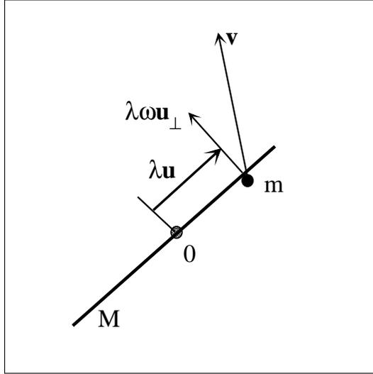
Fig. 1 – The needle and a bath particle in the plane:  $\mathbf{u}$  is a unit vector along the axis of the needle forming with  $\mathbf{u}^\perp$  an orthonormal system. The element of the needle at  $\lambda\mathbf{u}$  moves with linear velocity  $\lambda\omega\mathbf{u}^\perp$ . For a point of impact  $\lambda\mathbf{u}$  the pre-collisional relative velocity equals  $\mathbf{V} = \mathbf{v} - \lambda\omega\mathbf{u}^\perp$
