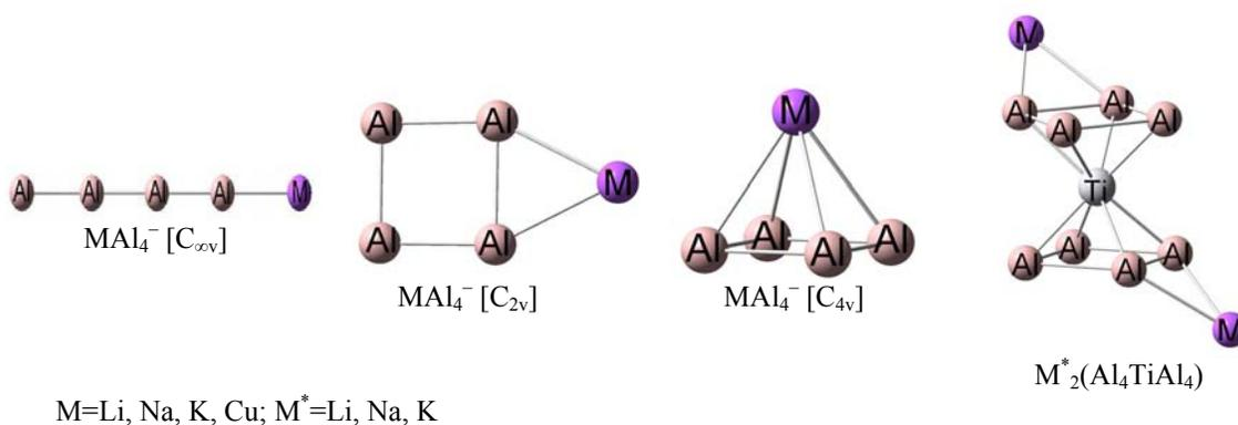
**Figure 2.** Optimized structures of various isomers of  $MAI_4^-$  ( $M=Li, Na, K, Cu$ ) and aromatic sandwich complexes  $M^*_2(Al_4TiAl_4)$  ( $M^*=Li, Na, K$ ).
