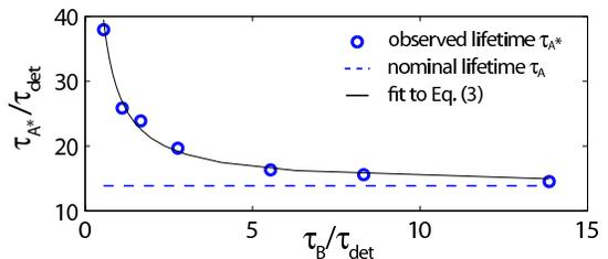
FIG. 4: Observed lifetimes  $\tau_{A^*}$  from a simulated process with  $\tau_A = 25 \mu\text{s}$  and  $\tau_B = 1$  to  $25 \mu\text{s}$ . The signals were filtered with  $f_c = 1 \text{ MHz}$  and processed with the Schmitt-trigger algorithm. From a fit (solid line) we find  $\tau_{\text{det}} = 1.8 \mu\text{s}$ . Because  $\tau_{\text{det}}$  represents the overall response of both the filter and the algorithm, it is not surprising to find  $\tau_{\text{det}} > 1/f_c$ .
