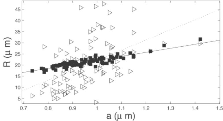
Figure 7: Best fit to the experimental data ( $\triangleright$ ) by a  $h(a)$  law for  $L_{\parallel} = 7 \mu\text{m}$  and  $\omega = 194 \text{ Hz}$ , as given by Eq. (24) ( $\blacksquare$  and best fit, straight line). The dotted line represent the best fit of the experimental data by a straight line (in the least-square sense), which we have added as a guide to the eyes.
