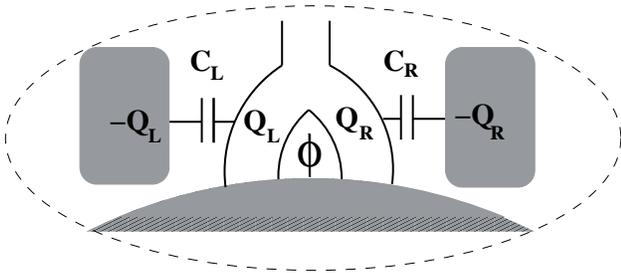
FIG. 3: Aharonov-Bohm loop capacitively coupled to external charged gates. The system as a whole (inside the dashed line; this includes the full cavity which we drew only partially) is electrically neutral, which does not prevent charge fluctuations in the arms of the loop to occur, provided they are compensated by fluctuations in the gates. The fluctuations in  $Q_L$  and  $Q_R$  induce fluctuations of the internal electric potential in the corresponding arm.
