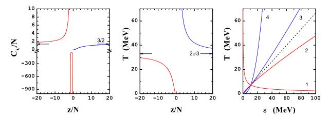
FIG. 1: The dependence of the heat capacity (left) and the temperature (center) on the specific  $\tilde{z} = z/N$  for the classical ideal gas of N nucleons at the values of the specific energy  $\varepsilon = 50$  MeV and the specific volume  $v = 3/\rho_0$ . The temperature as a function of the specific energy (right) for the different values of  $\tilde{z} = -1$ , -10, 10 and 1 (the curves 1, 2, 3 and 4, respectively) at  $v = 3/\rho_0$ . The dashed line corresponds to the Gibbs statistics.
