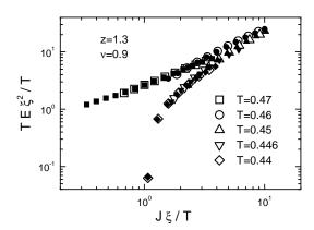
FIG. 3: Scaling plot of the nonlinear resistivity data for the smallest current densities near  $T_c=T_{ch}=0.455$  with  $\xi\propto |T/T_c-1|^{-\nu}$ . Open symbols correspond to L=128 and filled ones to L=180.
