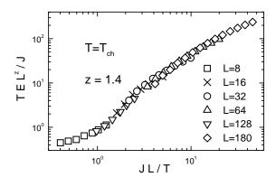
FIG. 5: Scaling plot of the nonlinear resistivity E/J at  $T_c=T_{ch}=0.455$  for different system sizes L.
