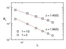
FIG. 6: Linear resistance as a function of system size at the critical temperatures  $T_c = T_{ch}$  for f = 1/2 and  $T_c = 0.887$  for f = 0. Power-law fits give estimates of the dynamic exponent
