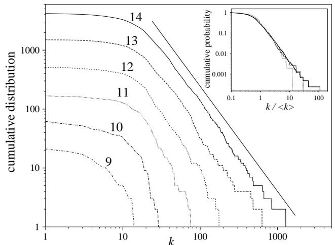
FIG. 3: The cumulative distribution for the number of nodes that have more than  $k$  connections. The curves correspond to clusters of different sizes, as labelled. An additional straight line with slope  $-(\gamma - 1)$ , where  $\gamma=2.78$ , has been plotted to emphasise the power law tail. In the inset the cumulative probability distribution for the 12-, 13- and 14-atom clusters is plotted against  $k/\langle k \rangle$ , to bring out the universal form of the distribution.
