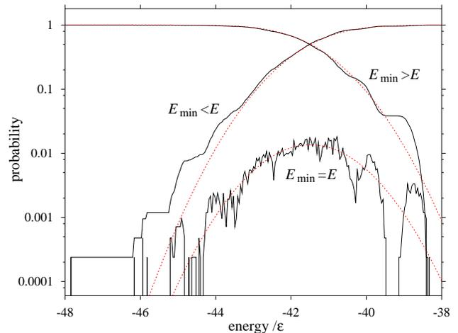
FIG. 5: (Colour online). (Cumulative) probability distributions for the energy of the minima for LJ<sub>14</sub>. The distributions are compared to Gaussian forms (dotted lines).
