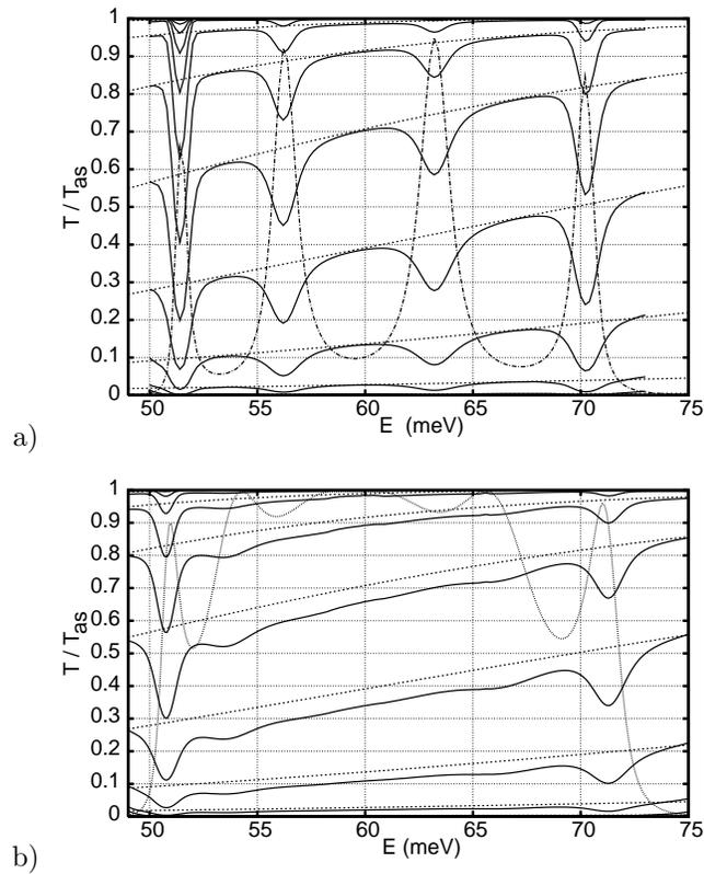
FIG. 9. Ratio  $T/T_{as}(E)$  with (solid line) and without potential (dotted line) for (a) five barrier periodic system and (b) with single-layer ARC added. The contours are plotted at intervals  $t = 2(1.5)14$  ps. Also shown (dotted) is the transmission  $T(E)$ , for reference.
