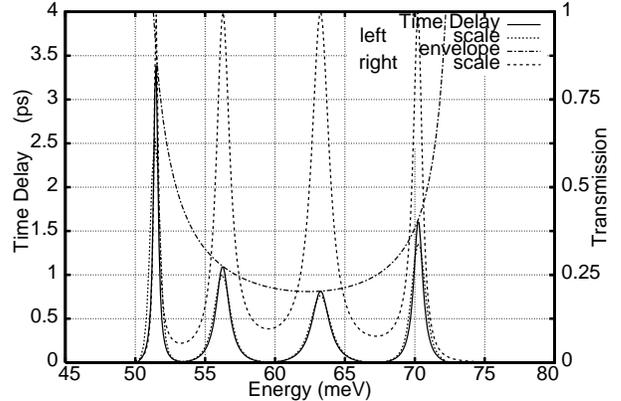
FIG. 11. Time Delay (solid line) computed from phase of  $t_N$ , and (dashed line) from the time-dependent calculation, just visible below the peaks. The dash-dot line is the locus, eq. 12. Also shown for reference is the transmission (dotted line).
