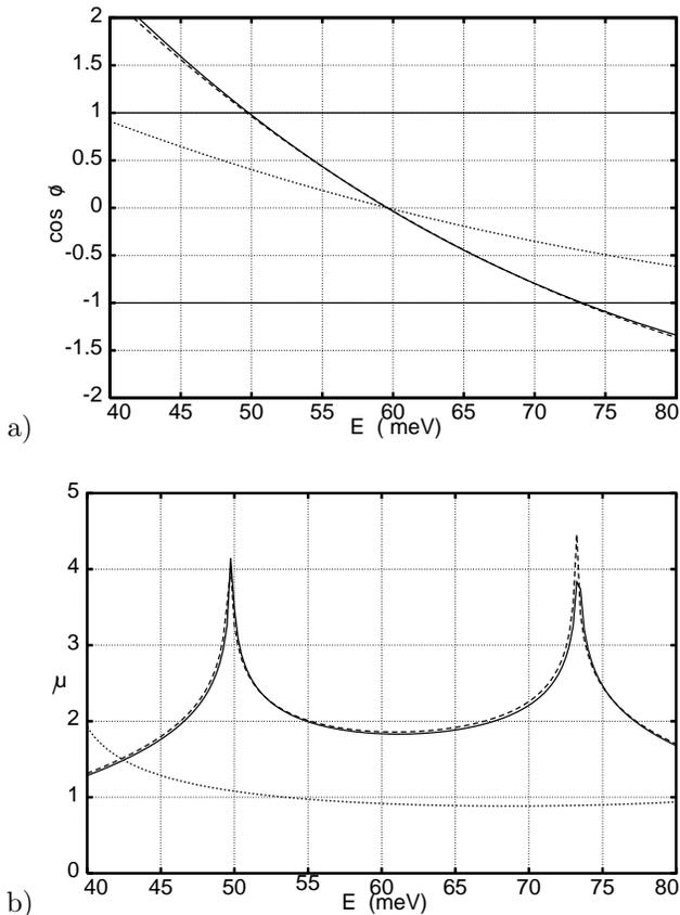
FIG. 2. Comparison of (a) Bloch phases of a square barrier cell (dash line) and our gaussian cell (solid line); also shown is  $\cos \phi_A$  of a single-cell ARC (dotted line). (b) same for impedance parameters  $\mu, \mu_A$ .
