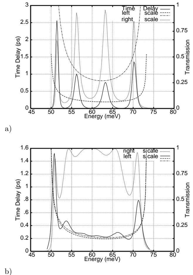
FIG. 10. Time delay (solid line) for electrons transmitted through (a) the five barrier periodic system and also (b) with single-layer ARC added. Also shown is the transmission  $T(E)$  (dotted line) for reference.
