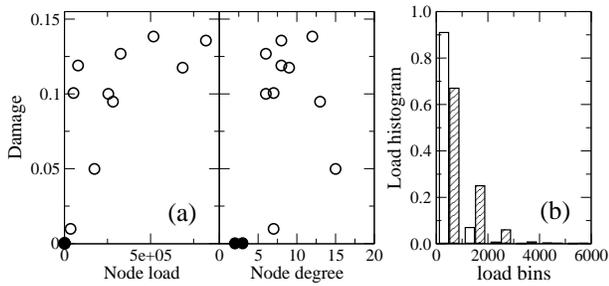
FIG. 5: (a) Correlation between node degree, load, and the efficiency loss its removal causes for 15 randomly selected nodes. The overload tolerance is  $\alpha = 1.2$ . The nodes causing no damage (filled circles) have low loads and degrees.(b) Load histogram for the generators (white bars) and transmission substations (dashed bars) whose removal does not cause any damage at  $\alpha = 1.025$ . A total of 639 generators and 476 transmission substations were included in this plot.
