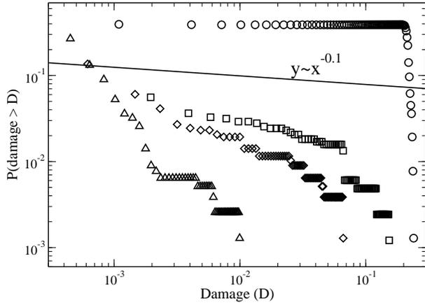
FIG. 3: Cumulative damage distribution for four different tolerance values,  $\alpha = 1.025$  (circles),  $\alpha = 1.2$  (squares),  $\alpha = 1.4$  (diamonds), and  $\alpha = 1.8$  (triangles). The continuous line indicates the cumulative distribution of disturbances on the power grid, i.e.  $P(d > D) = D^{\delta-1}$ , with  $\delta \simeq 1.1$ [19, 20].
