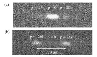
FIG. 3. Interference pattern of (a) phase shift =  $2n\pi$  and (b) phase shift =  $(2n+1)\pi$ . The absorption images are taken 10 ms after the recombining pulse.
