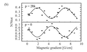
FIG. 4. Interference fringes after 1 ms propagation time in the waveguide with (a) the magnetic gradient turned for  $500 \, \mu s$  while the average separation of clouds is  $8.82 \, \mu m$  and with (b) the magnetic gradient turned for the same time while the average separation of clouds is  $6.94 \, \mu m$ .
