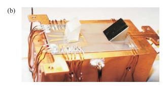
FIG. 1. (a) Schematic drawing of the atom chip (not to scale). The prism-shaped mirrors are integrated with microfabricated wires on an aluminum nitride substrate. The dimensions of the whole chip are 5 cm by 2 cm. (b) A photo image of the atom chip glued onto a copper holder.
