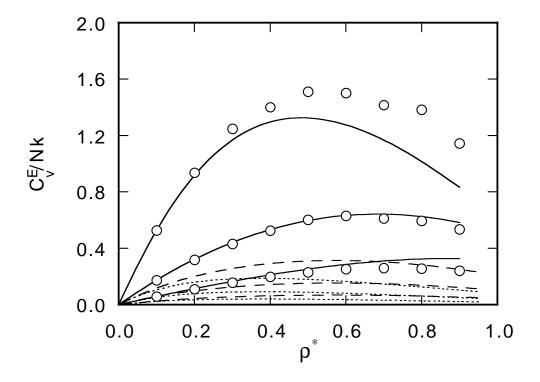
FIG. 1: Constant-volume excess heat capacity for a SW fluid with  $\lambda=1.1$  as a function of the reduced density  $\rho^*$ . Circles: simulation data from Table I for  $T^*=0.7$ ,  $T^*=1.0$ , and  $T^*=1.5$ , respectively, from top to down. Continuous curve: YAS model. Dashed curve: BH perturbation theory in the local compressibility approximation. Dotted curve: BH perturbation theory in the macroscopic compressibility approximation.
