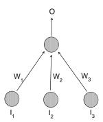
Fig. 2. A simple network containing four threshold units (three in the input and one in the output) for performing logical operations like AND, OR, NAND, etc.
