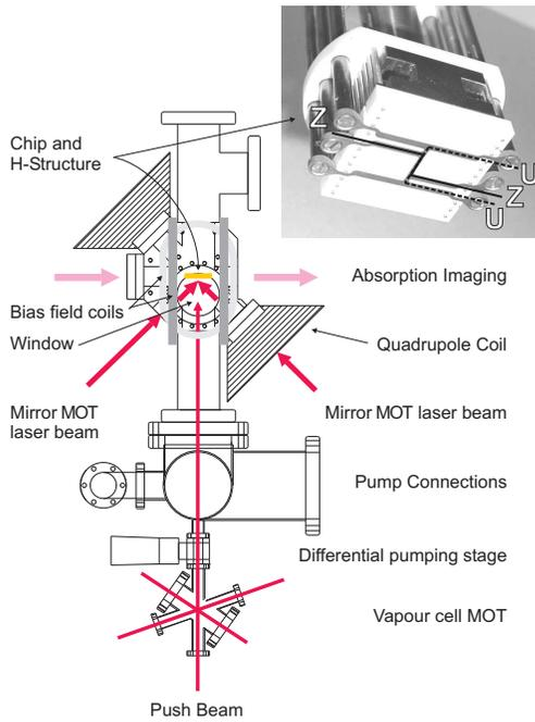
FIG. 1: Scheme of the experimental setup, showing the vacuum chamber, the quadrupole coils and the  $45^\circ$  laser beams for the mirror-MOT (see text). The inset shows the copper H-structure in the atom chip mounting (seen from below, atom chip not mounted). The current paths for the U- and the Z-trap are indicated.
