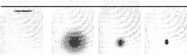
FIG. 4: Bose-Einstein condensation is observed in absorption images taken at different final RF-frequencies  $\nu_f$ . From left to right: atoms in the trap,  $\nu_f = 800$  kHz, expanded clouds after 15 ms time-of-flight with  $\nu_f = 800$  kHz (thermal cloud),  $\nu_f = 650$  kHz (bimodal cloud) and  $\nu_f = 630$  kHz (pure BEC), respectively. Each image size is  $\sim 1.8 \times 2.3$  mm. The surface of the atom chip is indicated at the top of the figure.
