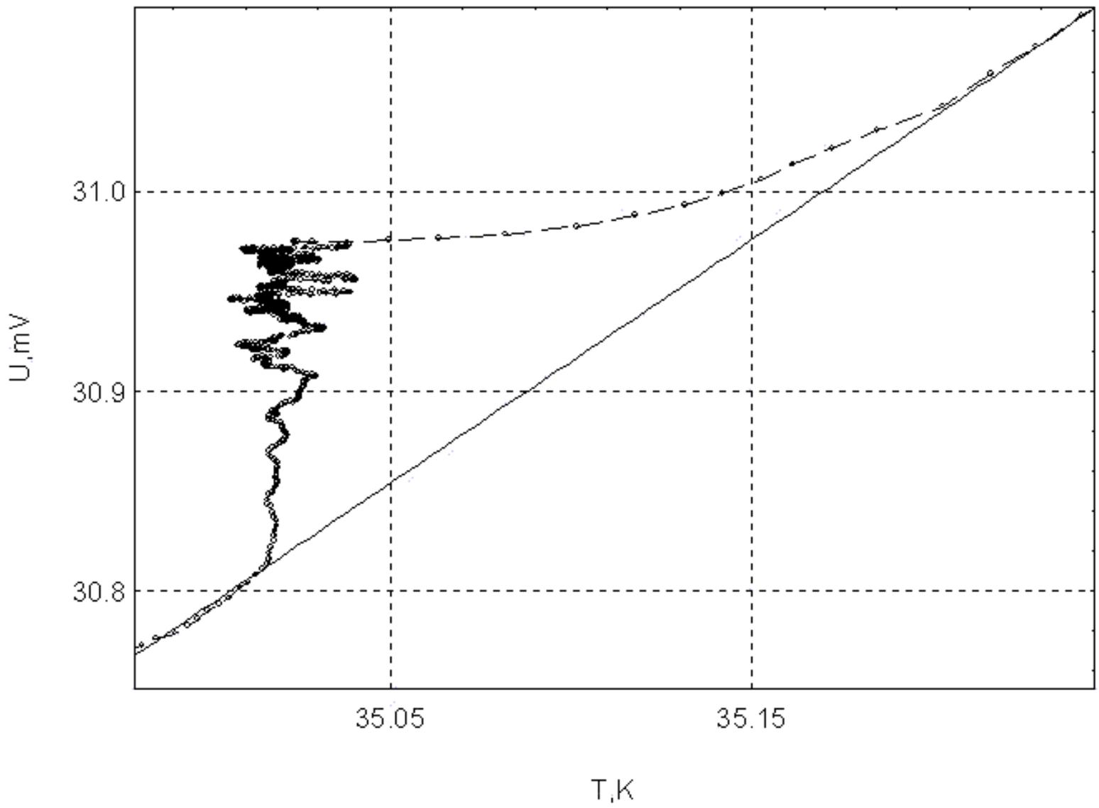
Fig.3. Behaviour of induction  $B(T)$  after creep at a fixed temperature during  $10^4$  s.
