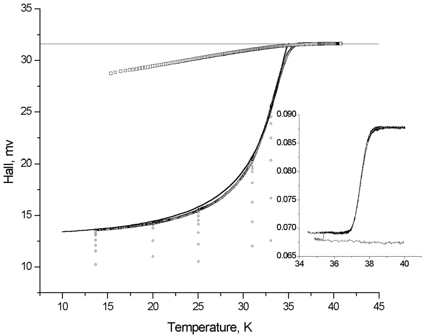
Fig.1. Temperature dependence of MgB<sub>2</sub> sample induction in field  $\approx 0.2$  T.
