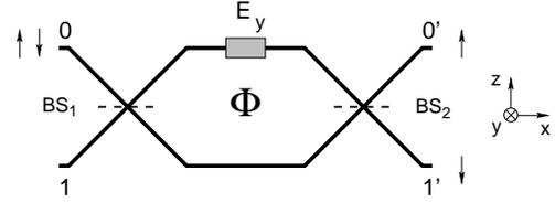
FIG. 1: A sketch of the proposed spin polarizing beam splitter. Unpolarized spins are injected in mode 0; the  $0'$  ( $1'$ ) output mode contains only spin up (down) polarized electrons.  $BS_{1,2}$  are two beam splitters; a magnetic flux  $\Phi$  is applied through the interferometer generating an Aharonov-Bohm phase. An electric field  $E_y$  is applied locally on the upper arm (the 1-mode) generating a Rashba phase (the gray box).
