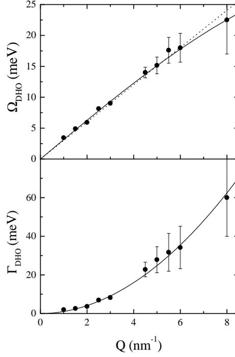
FIG. 2.  $Q$ -dependence of the sound frequency and attenuation. Upper panel: experimental sound dispersion (full dots) and best fit through a sine function (full line). The adiabatic sound speed, measured by ultrasounds, is also reported (dotted line). Lower panel: Acoustic attenuation as determined by the Brillouin linewidth (full dots). The solid line is a power law fit to the experimental data and gives  $\Gamma_{DHO} = 1.05Q^{1.96}$
