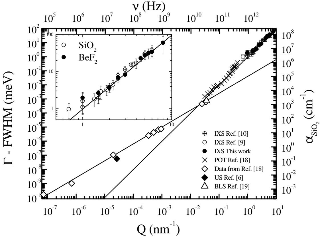
FIG. 4. Sound attenuation of  $\text{BeF}_2$  and  $\text{SiO}_2$  determined with different techniques (the right scale is for  $\text{SiO}_2$  data only). The full lines are  $Q^2$  and  $Q^{1.3}$  power laws. The inset details the IXS frequency window
