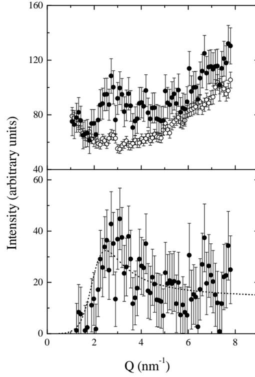
FIG. 3. Fixed energy IXS  $Q$ -scan. Upper panel: inelastic ( $I(Q, E = 7 \text{ meV})$ , full dots) and elastic ( $I(Q, E = 0 \text{ meV})$ , open dots). Lower panel: genuine inelastic signal determined as the difference of the above reported scans (normalized according to Ref. [17]), compared to a theoretical DHO with parameters determined as discussed in the text.
