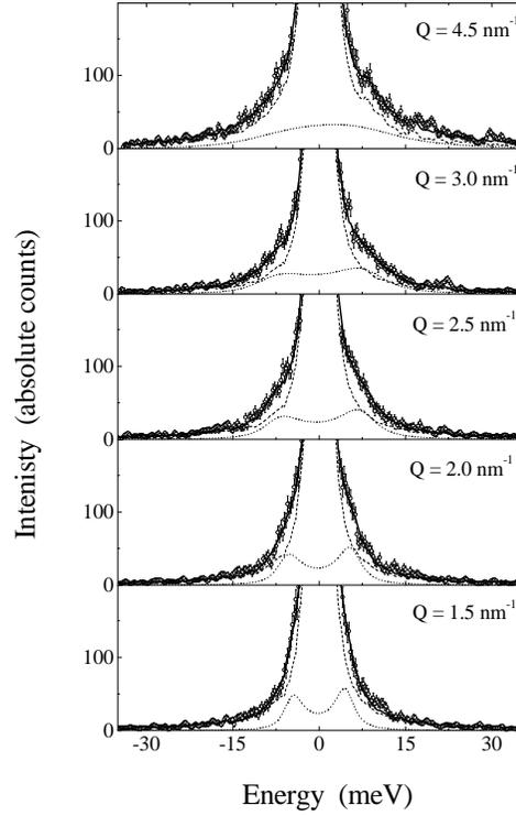
FIG. 1. Selected IXS energy spectra of the  $\text{BeF}_2$  glass at room temperature and fixed values of the exchanged wavevector (open dots  $\circ$ ). The solid lines represent the best fits with Eq. 7, while dashed and dotted lines account for the elastic and inelastic contributions, respectively, as determined by the fitting procedure.
