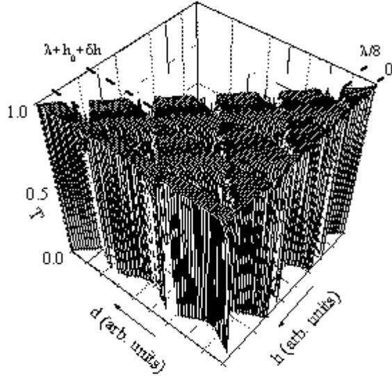
FIG. 3. Spin-down transmission of an array of five stub tuners as a function of the stub length  $h$  and stub shift  $d$  when only spin-up electrons are injected. Cross sections along the dashed lines are shown in Fig. (4).
