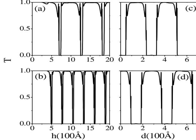
FIG. 4. Two-dimensional cross section of Fig. (3) in the transmission  $T$  vs stub length  $h$  for fixed  $d$  ( $d = 0$  in a) and  $d = \lambda/8$  in b) ) and vs stub shift  $d$  for fixed  $h$  ( $h=1289.5\text{\AA}$  in c) and  $h=1568.5\text{\AA}$  in d) ).
