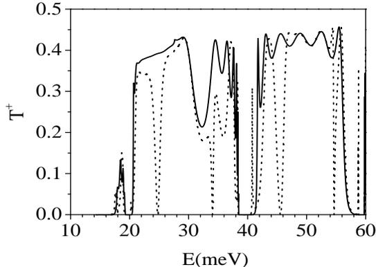
FIG. 7. Spin-up transmission  $T^+$  versus electron energy  $E$  for a periodic array of seven units (solid line) and for the same structure with the central (fourth) unit replaced by a defect unit.
