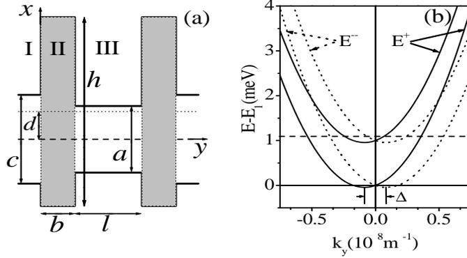
FIG. 1. (a) Schematics of a stub tuner with two units. The waveguide segment between the two stubs (shaded regions of width  $b$ ) has length  $l$  and widths  $a$  and  $c$  as indicated. The asymmetry parameter  $d$  is the distance between the lines, along the  $y$  axis, that bisect the main waveguide and the stubs as indicated. (b) Dispersion relation for a waveguide based on Eq. (9). The horizontal dashed line indicates the four possible values of the wvector for the same energy  $E$ .
