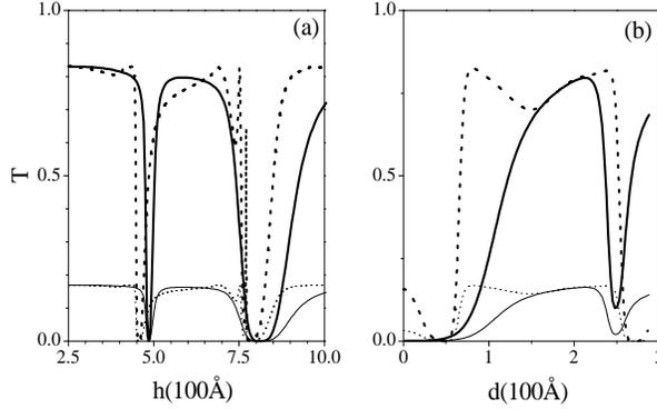
FIG. 5. Transmission as a function of the stub length  $h$ , for symmetric double stubs (a), and of the stub shift  $d$  for asymmetric double stubs (b). The thin and thick solid curves show, respectively, the spin-up and spin-down transmission for Gaussian shaped stubs. The thin and thick dotted curves show the corresponding results for rectangular stubs with parameters  $a = 250\text{\AA}$ ,  $b = 290\text{\AA}$ ,  $L = 360\text{\AA}$ .
