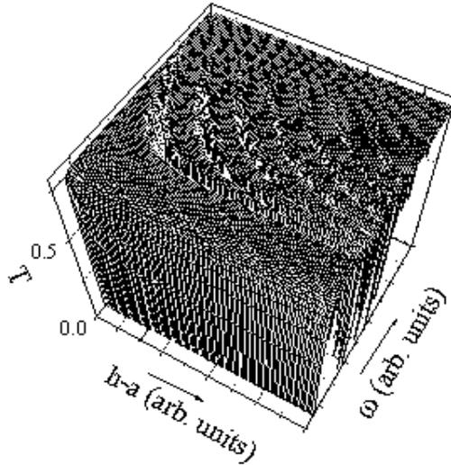
FIG. 2. Three-dimensional illustration of transmission  $T$  versus electron energy and stub arm length  $h - a$  of a *symmetric* stub tuner.
