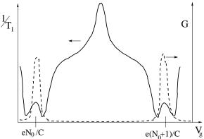
FIG. 2. Sketch of the predicted NSR dependence on  $V_g$  in the presence of SOC. Dashed line shows the linear conductance through the dot.
