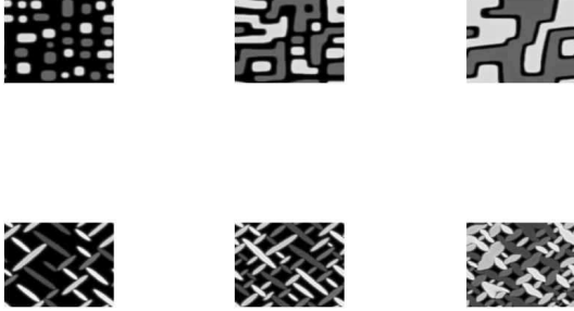
FIG. 2. : Phase separation final state on a (001) Copper crystal surface with \Lambda = 40 \text{ mJ/m}^2 (defined in the text) for a C2X2 (first row) at \theta_0 = 0.25 (on the left), \theta_0 = 0.5 (in the middle), \theta_0 = 0.75 (on the right hand side) and for a P2X1 (second row) with \mu = 0.9\Lambda at \theta_0 = 0.38 (on the left), \theta_0 = 0.5 (in the middle) and \theta_0 = 0.75 (on the right hand side). The gray scale enhances the different variants of the layer structures. The direction [010] is indicated.
