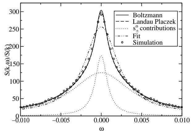
FIG. 2: The central part of the spectrum in the Boltzmann approximation, the Landau-Placzek approximation, the  $s_{\pm}^{\circ}$  contributions are shown separately. The system parameters are  $\theta = 0.1$ ,  $\rho = 6.5$ ,  $P_r = 0.05$ ,  $k_x = 4 \times 2\pi/512$ . The wavevector  $\mathbf{k}$  and frequency  $\omega$  are given in reciprocal lattice and time respectively.
