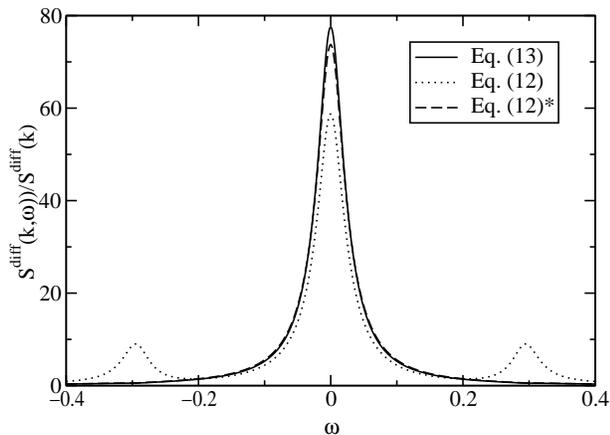
FIG. 3: A diffusive spectrum based on the different possible choices for the density difference. The curve labeled by \* is corrected by subtracting the propagating part. The system parameters are  $\theta = 0.05$ ,  $\rho = 10.0$ ,  $\rho_r/\rho = 0.15$ ,  $k_x = 20 \times 2\pi/512$ . The wavevector  $\mathbf{k}$  and frequency  $\omega$  are given in reciprocal lattice and time respectively.
