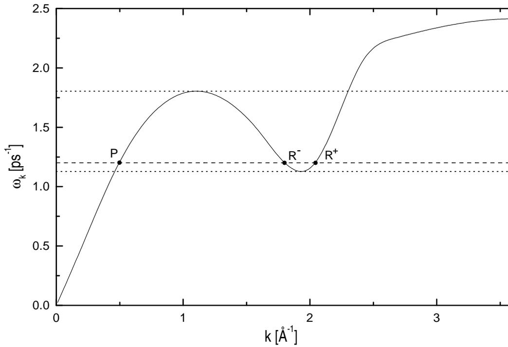
FIG. 1. Dispersion curve for elementary excitations in helium II (from Ref. 22). The dotted lines separate the regions where the equation  $\omega_q = \omega_k$  changes its number of solutions. The points  $P$ ,  $R^-$  and  $R^+$  on the dashed line illustrate about possible vortex-induced qp transitions.
