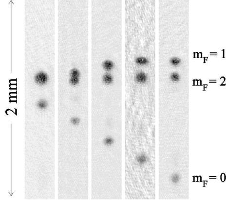
*Figure 1.3* Time of flight images of multiple condensates produced by a rf pulse. Taken after 15 ms of free fall, the pictures refer to different evolution times  $\Delta t$  in the magnetic trap, respectively 2,3,4,5 and 6 ms. The  $m_F = 2$  condensate is below the center of oscillation of the  $m_F = 1$ , opposite to what one expects considering the gravitational sagging. This can be explained by the presence of a gradient during the switching off of the magnetic field
