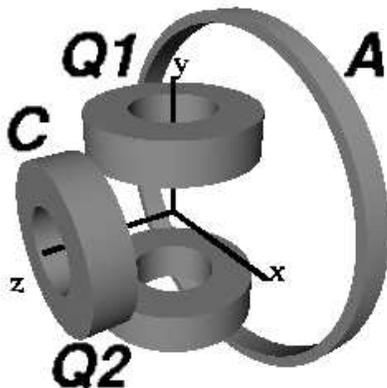
*Figure 1.1* 4-coils magnetic trap: Q1 and Q2 coils produce the quadrupole field, the curvature coil (C) provides the axial confinement and the antibias coil (A) reduces the bias field thus increasing the radial confinement.
