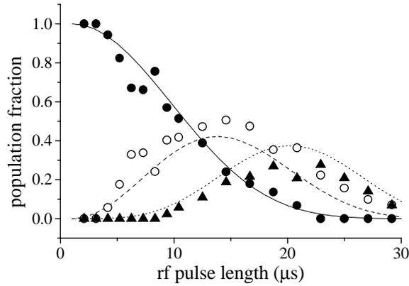
Figure 1.4 Measured population fraction of  $m_F = 2$  (solid circle),  $m_F = 1$  (open circle) and  $m_F = 0$  (triangle) states as a function of rf pulse duration. The curves correspond to the calculated Rabi oscillations of the relative population in  $m_F = 2$  (solid line),  $m_F = 1$  (dashed line) and  $m_F = 0$  (dotted line).
