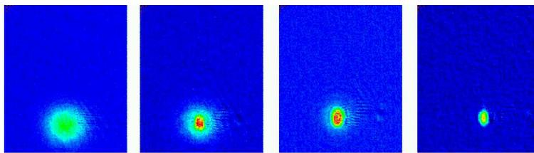
*Figure 1.2* Absorption imaging picture of the atomic cloud after a time of flight of 20 ms. From the left to the right the rf ramp was stopped respectively at 0.94 MHz, 0.92 MHz, 0.90 MHz and 0.88 MHz. The symmetric expansion in the first image is typical of a thermal cloud. By further evaporation the high density peak characteristic of the condensate emerges, finally giving rise to a pure condensate.
