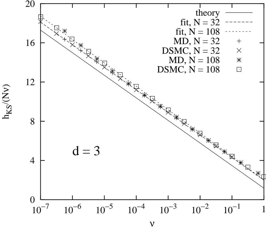
FIG. 2. A plot of the results for the KS entropy per particle for a dilute gas of three-dimensional hard balls, as a function of the collision frequency  $\nu$  in units of  $\sqrt{\frac{3}{2}k_B T}/(ma)$ . The solid line is the result given in Eq. (32), the data points are results of Dellago and Posch and the dashed curves are fits. The notation is the same as in the previous figure.
