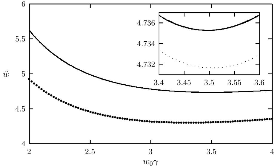
FIG. 3. Several approximations for the function  $\tilde{w}$ . A  $1 \times 1$  truncation of the matrices yields the dotted curve. The solid curve results from the  $3 \times 3$  matrices. As the difference is so small, only the blow-up in the inset can show the  $2 \times 2$  results separately as the curve of points.
