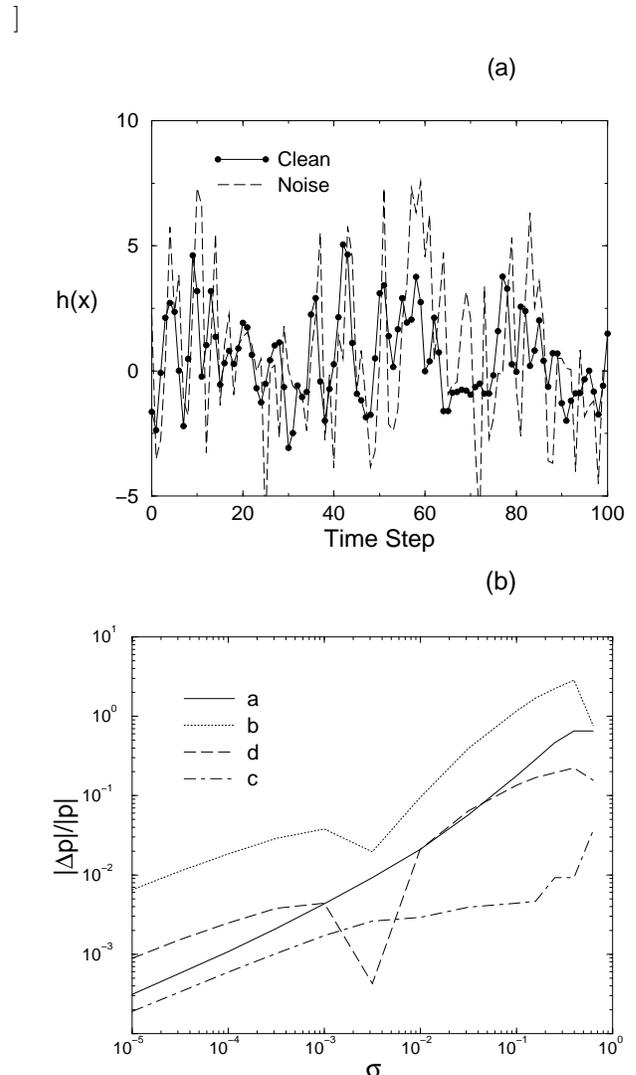
FIG. 4. The hyperchaotic generalized Rössler model. (a) Short samples of the time series used in the numerical experiments. The noisy time series represents 0 dB noise. (b) The relationship between the relative error in the parameter estimates and the size of the noise. Here,  $\Delta \mathbf{p} = \hat{\mathbf{p}} - \mathbf{p}^*$ .
