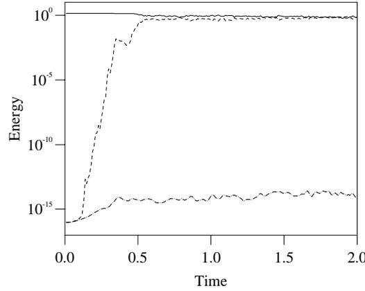
Fig. 3. – Ideal case: kinetic energy (continuous line) and magnetic energy (dashed line) versus time for the FS model; magnetic energy (dot-dashed line) versus time for the B model.
