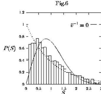
FIG. 6. The nearest-neighbor level spacing distribution  $P(S)$  is shown for  $\bar{v}^{-1} = 0$  in case of the scatterer being located at a generic position in the rectangular solid. The statistics are taken within the eigenvalues between  $z_{100} = 415.81$  and  $z_{3100} = 3503.68$ . The solid (dotted) line is the Wigner (Poisson) distribution.
