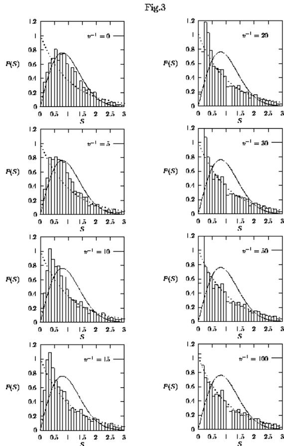
FIG. 3. The nearest-neighbor level spacing distribution  $P(S)$  is shown for various values of  $\bar{v}^{-1}$  in case of the scatterer being located at the center of the rectangular solid. The statistics are taken within the eigenvalues between  $z_{100} = 1307.95$  and  $z_{3100} = 12932.70$ . (The eigenvalues are numbered by taking into account only the eigenstates with even parity in each direction.) The solid (dotted) line is the Wigner (Poisson) distribution.
