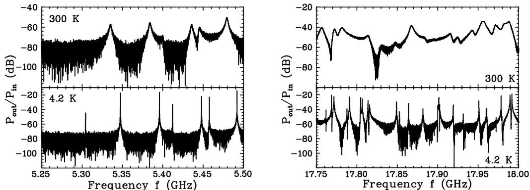
Fig. 1: Comparison of the normal conducting (upper part, at 300 K) and the superconducting (lower part, at 4.2 K) transmission spectrum of the  $\lambda = 0.15$  billiard for two different frequency ranges.
