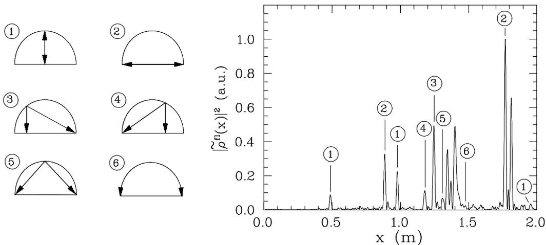
Fig. 3: On the left side the shortest periodic orbits for the classical billiard ( $\lambda = 0.3$ ) are sketched. On the right side the Fourier Transform of the fluctuating part of the level density is shown. The encircled numbers above the peaks label the classical periodic orbits.
