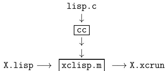
6. `clispm.m` is a *Mathematica* program serving as a driver for a *C* program that simulates a *LISP* interpreter running on a register machine. `clispm.m` converts an `X.lisp` input file into an `X.cmrun` output file.
