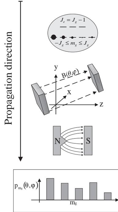
FIG. 2. Setup of a Stern-Gerlach experiment with an additional homogeneous magnetic field  $\vec{B}(\theta, \varphi) = |B| \vec{n}(\theta, \varphi)$  inducing spin precession around the axis  $\vec{n}(\theta, \varphi)$
