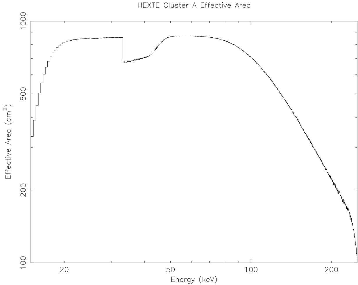
Fig. 5.— The HEXTE effective area versus energy for cluster A. The reduction at lower energies is due to photoelectric absorption in the housing above the detector, while the reduction at higher energies is due to the finite NaI(Tl) thickness. The sharp drop and smooth recovery near 30 keV is due to the change in photoelectric cross section at the K-edge of iodine and the onset of K-escape losses.
