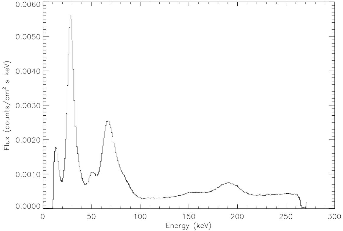
Fig. 6.— The HEXTE background for a single detector plotted versus energy. Background lines due to activation of the iodine by cosmic and trapped radiation are evident at 30, 55, 66, and  $\sim 190$  keV, as are the  $K_{\alpha\beta}$  lines at 74 and 85 keV from fluorescence of the lead collimator. The data are from a 7.5 hour observation of blank sky fields.
