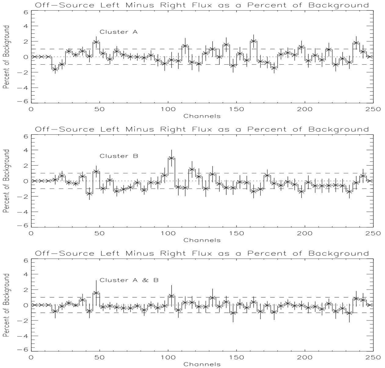
Fig. 9.— The net counting rate histogram of the difference of the two off-source positions for each cluster and their sum during the MCG 8-11-11 observation. One percent of the total off-source flux is shown by pairs of horizontal dashed lines for comparison. “Left” and “Right” correspond to the plus and minus directions of the off-source viewing.
