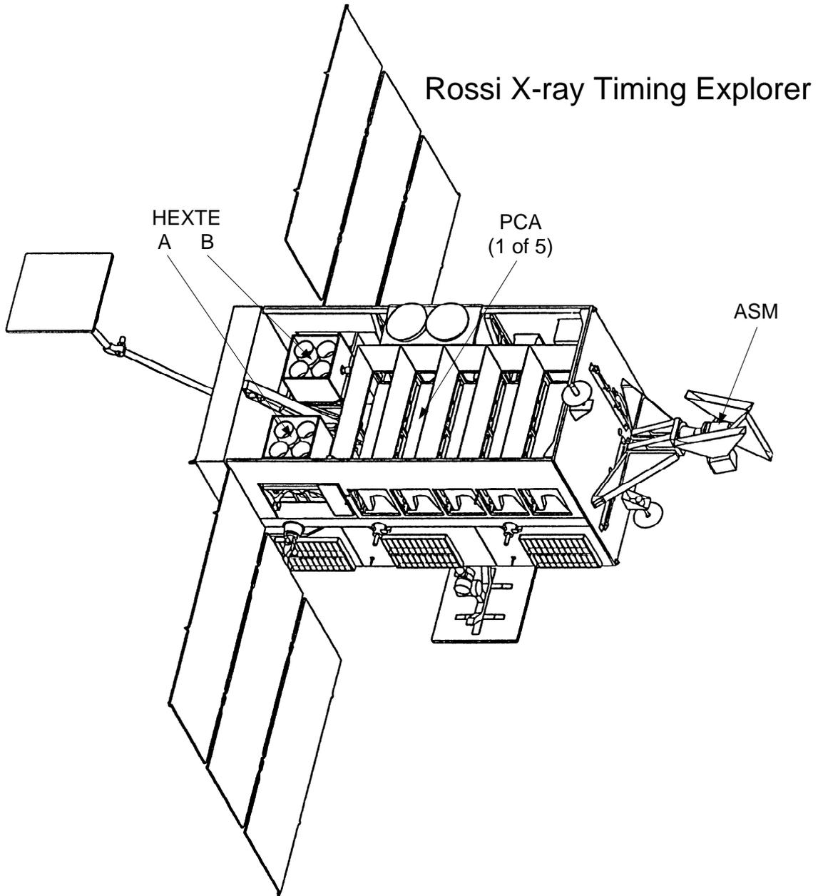
Fig. 1.— The *RXTE* spacecraft viewed from above to reveal the scientific instruments. The five PCA proportional counters and the two HEXTE clusters are shown in relation to the rest of the spacecraft components, such as the two high gain antennae for communications with the ground via the Tracking and Data Relay Satellite System, the two solar-power arrays that can rotate to face the sun, and the ASM on the end with clearance to view the sky.
