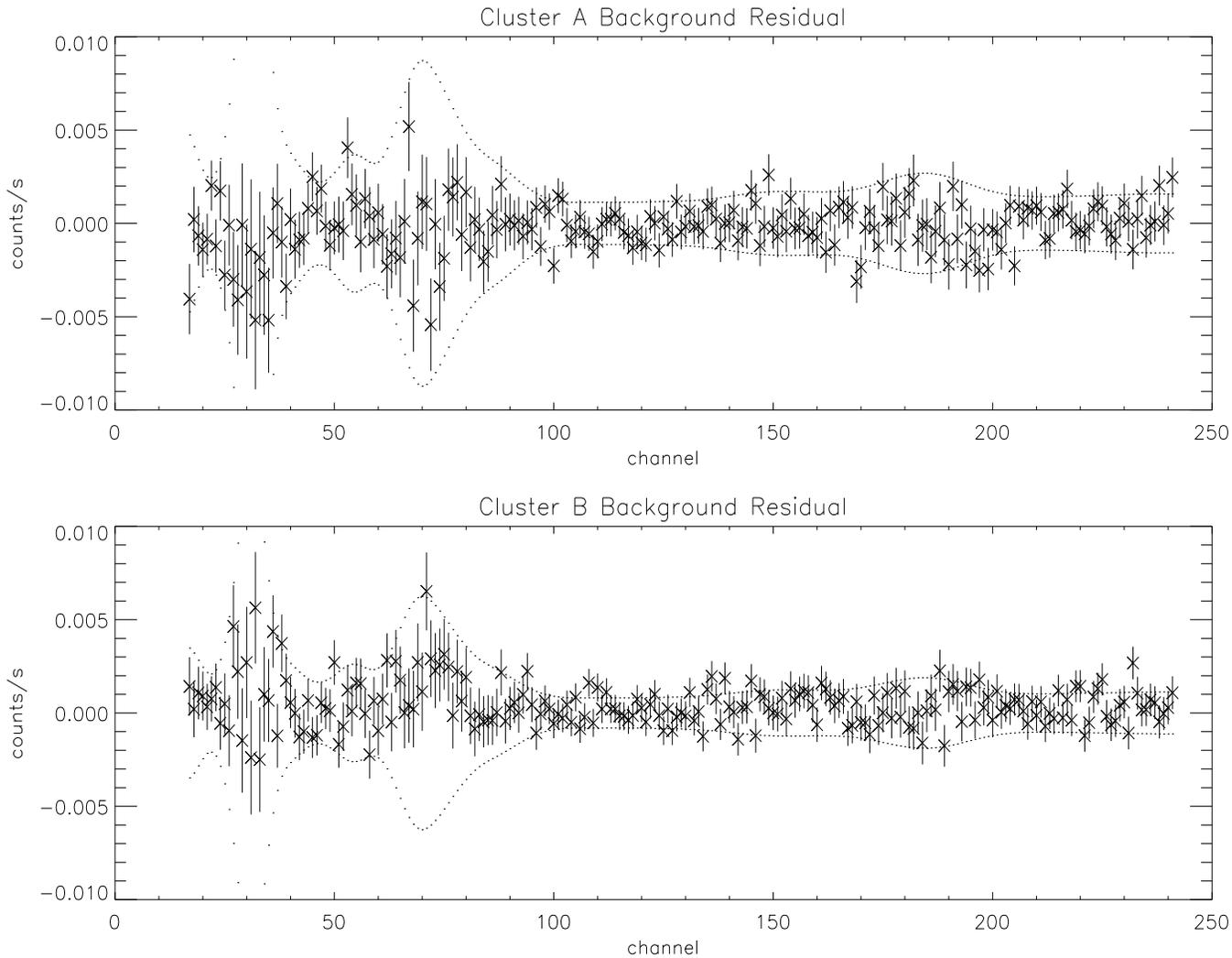
Fig. 10.— The net off-source counting rate histogram versus pulse height channel for a  $5 \times 10^6$  s accumulation of observations with greater than 50 ks duration for the two HEXTE clusters. The detector gain is approximately one keV per channel, and the energy range covered is 15–240 keV. The dotted lines represent  $\pm 0.5\%$  of the background per channel.
