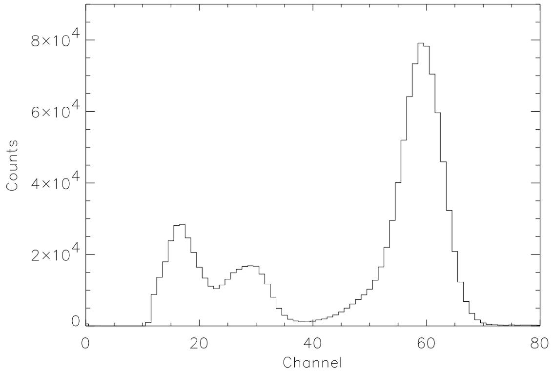
Fig. 3.— Calibration histogram of the HEXTE  $^{241}\text{Am}$  gain control source. The data were accumulated over one day on 10 January 1997. The 60 keV gamma-ray line, the complex of Np L de-excitation lines around 17 keV, and the K-escape lines near 30 keV are evident. Each channel corresponds to approximately 1 keV.
